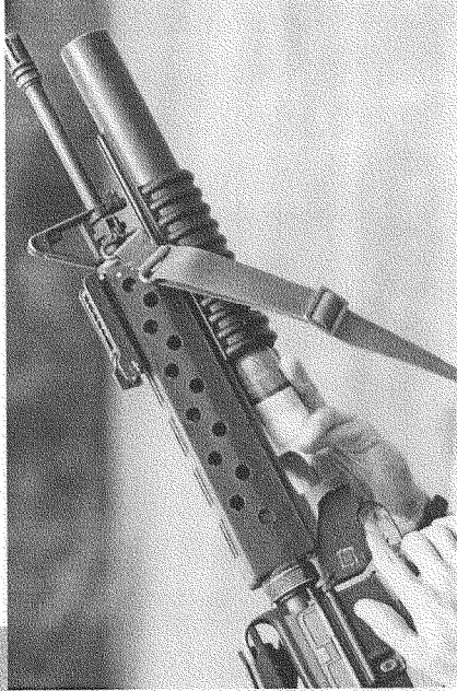
M7 66 Millimeter Grenade Launcher Attachment for M16 rifle
