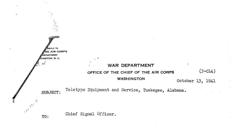
1. It is requested that two model 15 teletype machines be shipped to the Air Corps Flying School, Tuskegee, Alabama, marked "For Air Corps Weather Station". It is desired that these machines be installed in the weather station; and that they be connected, one to Circuit 4, Schedule A, and one to Schedule C, for receiving only.
